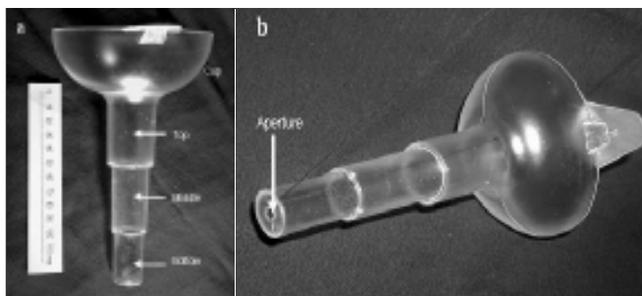
Figure 1: Photographs of the device showing a, the 3-chamber design and b, the 4.6 mm aperture
